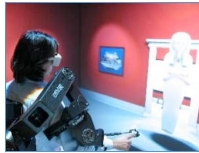
Figure 4: A user wearing the specially designed Haptic Interface in the form of an exoskeleton in the Museum of Pure Form
